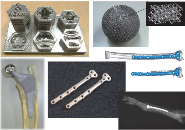
Fig. 9 Various metal AMed products. It is capable of fabricating complex external and internal geometry, mesh structure, solid body with customized external geometry, and mesh on solid surfaces, reflecting 3D design on CAD.
