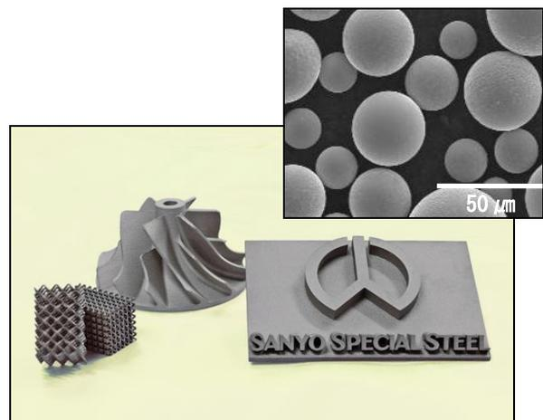
■ Top: Extremely spherical metal powder (electron microscope image)
