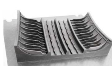
The 3D molding using the metal powder can integrally mold the composite shape (Tire Mold)
