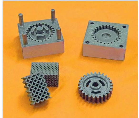
【Examples of moldings by additive manufacturing】
