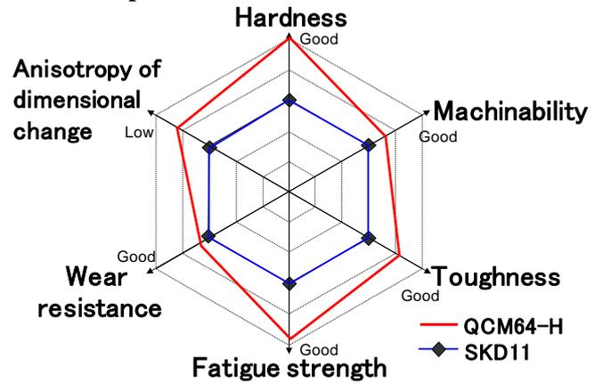
(2) Displays outstanding performance under the heat treatment conditions as general purpose cold-work tool steel
