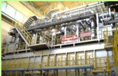
Energy-saving heating furnace that uses regenerative burners
