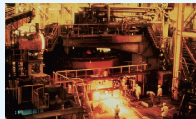
150-ton electric arc furnace (1982)
