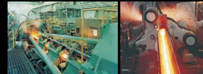
Assel tube rolling mill
