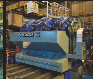
Reducing and sizing block [RSB]
