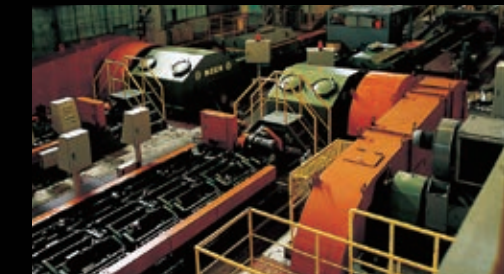
Cold pilgering mill
