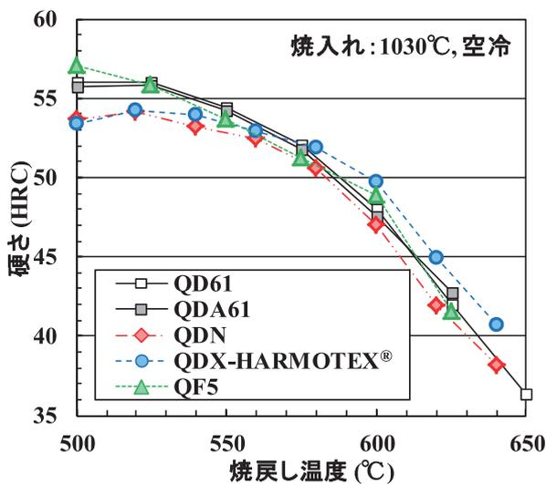
図2 QD61, QDA61, QDN, QDX-HARMOTEX<sup>®</sup>, QF5の焼入焼戻し硬さ
