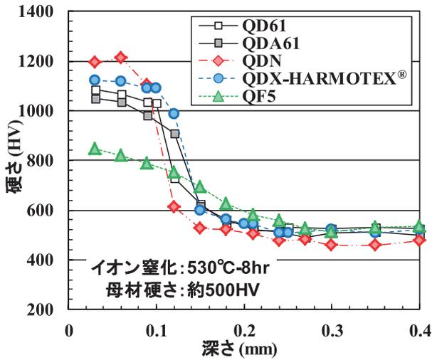
図5 QD61, QDA61, QDN, QDX-HARMOTEX®, QF5の窒化特性
