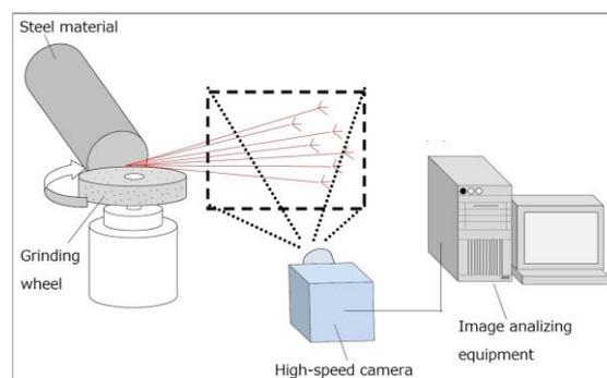
Figure 2: Schematic layout of the test machine
