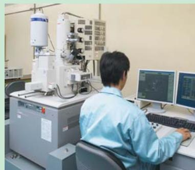
High-resolution field emission scanning electron microscope
