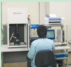
Ultrasonic fatigue testing equipment
