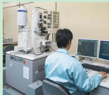
High-resolution field emission scanning electron microscope
