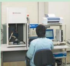
Ultrasonic fatigue testing equipment
