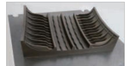
Example of molding by 3D printing: Tire mold
