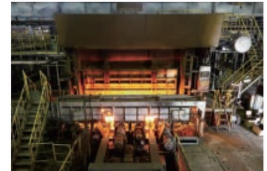
A heating furnace with energy-saving burners
