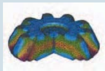
Strain distribution of a cold forged gear
