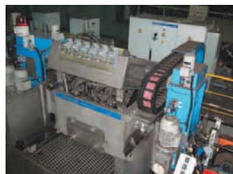
Phased-array ultrasonic inspection machine
