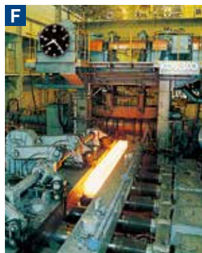
[Cogging mill] Blooms are rolled to create interim products called billets.
