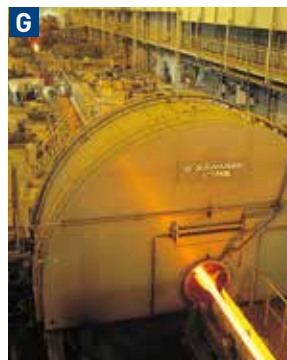
[Billet rolling mill(PSW)] We efficiently manufacture billets using the three-roll method, which offers superior rolling capability. Sizes can also be changed easily.
