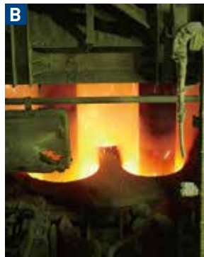
[Ladle furnace] Impurities are removed from the liquid steel and alloy iron is added. Finally, components are adjusted to determine the special characteristics of the steel.
