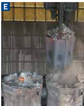
[Ingot caster] This casting method hardens liquid steel inside the die. Our 60-t steelmaking plant is equipped with both ingot casting and completely vertical type bloom caster.
