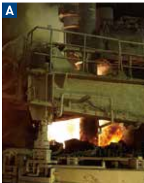
[Electric arc furnace] Arc discharge and auxiliary burners are used to heat furnaces to high temperatures (1,500-1,600°C) and melt iron scrap down to liquid steel.
