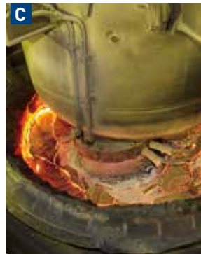
[RH vacuum degasser] Liquid steel is recirculated in a vacuum to remove unnecessary gas components and further increase the cleanliness of the steel.
