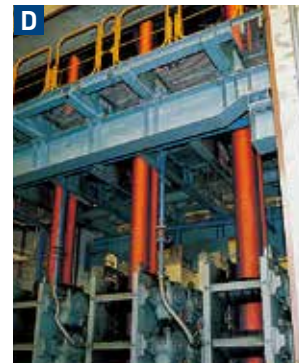
[Continuous caster] Liquid steel is hardened and formed into blooms (slabs). Sanyo Special Steel has introduced completely vertical type bloom casters, which offer superior quality.
